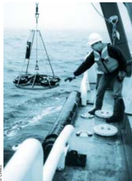
A Van Veen bottom sampler is lowered during the Pacbaroness expedition.
