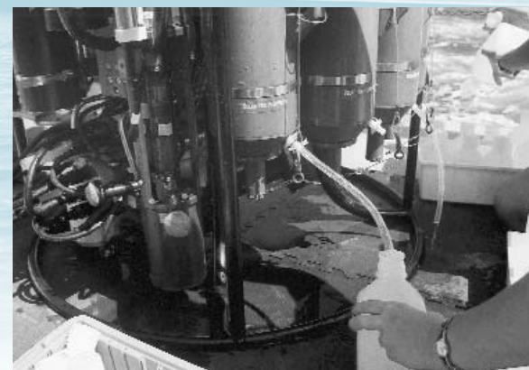
Scientists from the Plumes and Blooms project collect water samples from their 450-pound instrument package, which is deployed using the R/V Shearwater’s hydraulic A-frame and winch.
