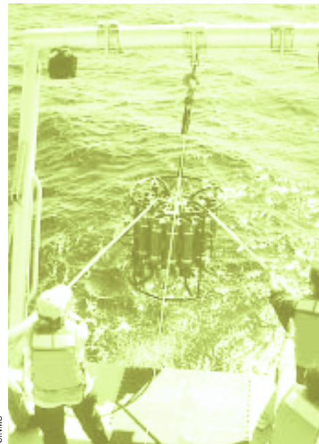
Plumes and Blooms scientists use an instrument called a CTD to measure conductivity, temperature, and depth at various points in the water column.
