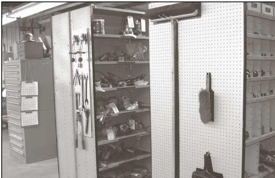
Central Tool Room after painting and shadow boarding
