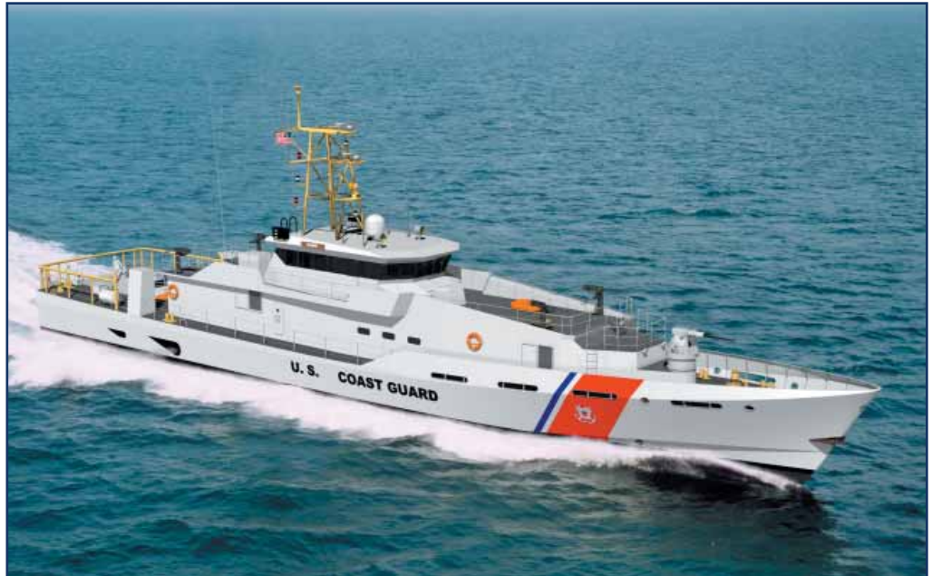
The Sentinel-class Fast Response Cutters will replace the Coast Guard’s aging 110-foot patrol boats. The Sentinel is a 153-foot vessel capable of more than 28 knots. The Coast Guard plans to acquire as many as 34 FRCs of the Sentinel-class design, and may consider acquiring 24 more of this or another design, for a total force structure of 58 FRCs. (Graphic by Bollinger Shipyards, Inc.)
