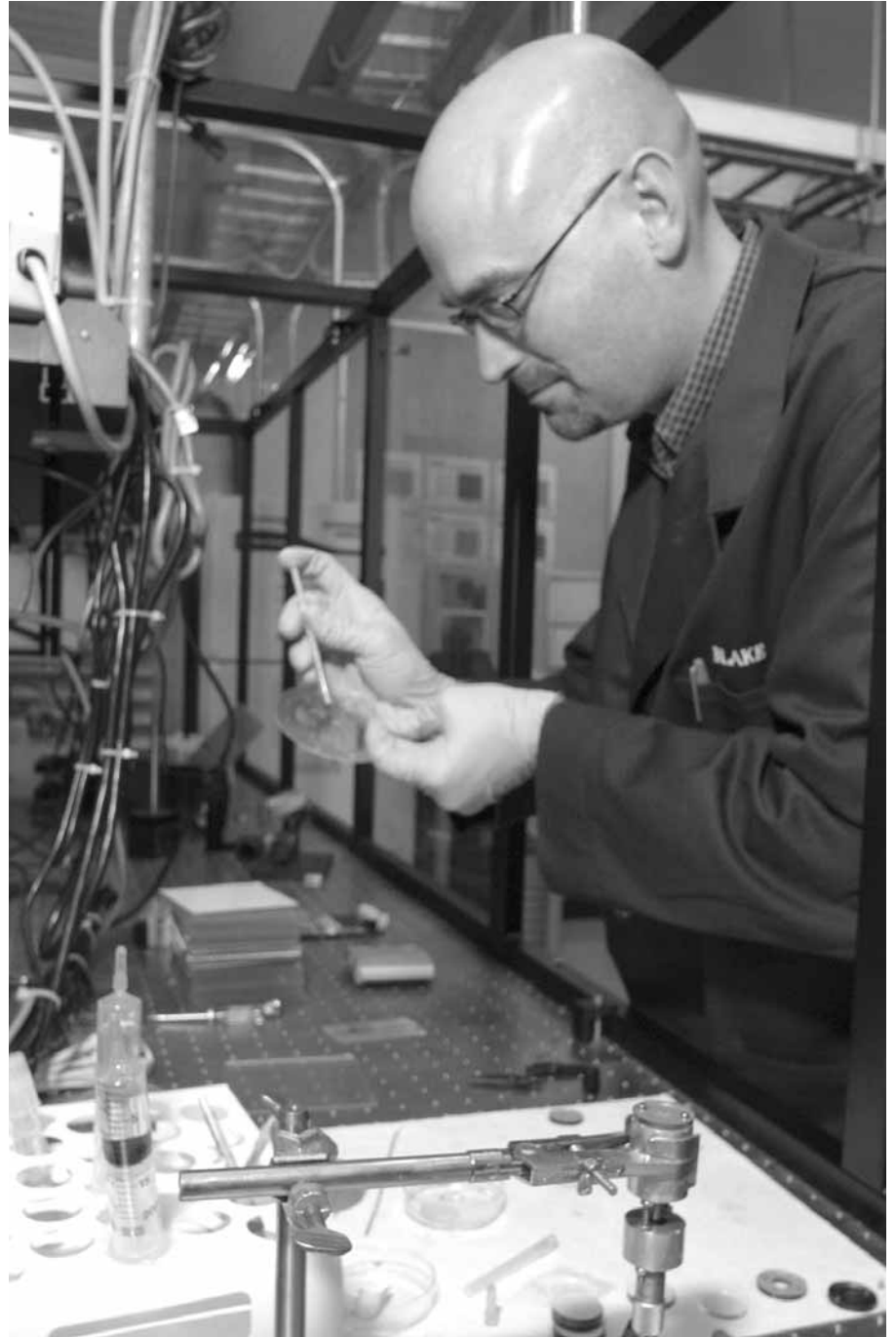
BLAKE SIMMONS prepares the iDEP polymer microfluidic device for use as a particle concentrator. iDEP can deliver detectable amounts of material in small sample volumes, eliminating any need for overnight culturing and significantly speeding up overall water analysis. (Photos by Bud Pelletier)
