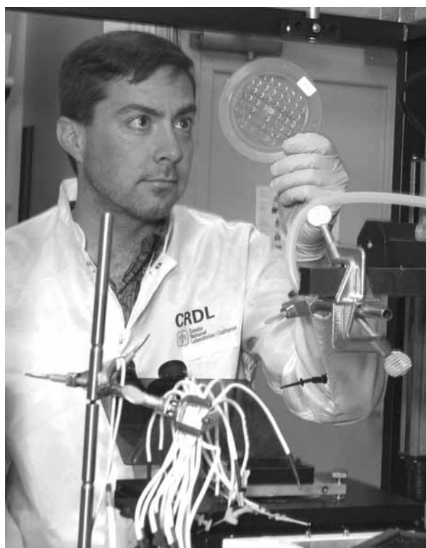
ERIC CUMMINGS visually inspects an iDEP device for proper alignment before evaluating it with a fluorescent microscope. Among other potential applications, iDEP may allow for protein isolation and concentration, sample concentration and focusing, analytical chemistry, and mass spectrometry for proteomics and drug discovery.
