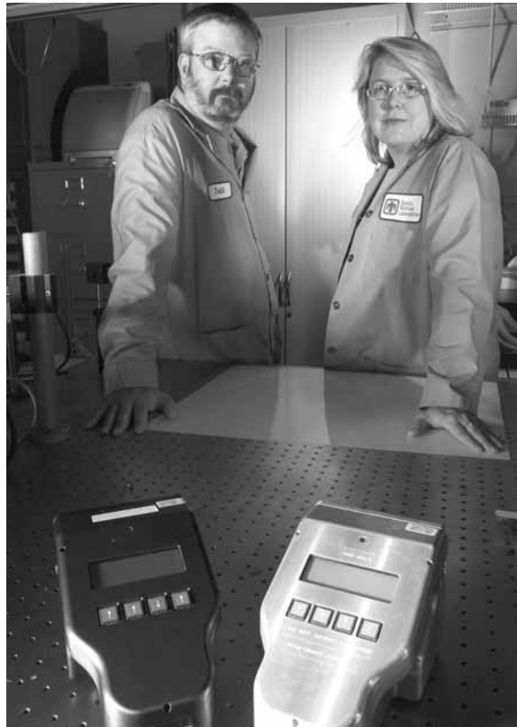
SANDIA RESEARCHERS Todd Lane and Victoria VanderNoot are leading an effort to detect deadly toxins from HABs. The project employs laser-induced fluorescence and other separation methods inherent in Sandia’s \mu ChemLab™ device, examples of which are seen here. (Photo by Jeff Shaw)
