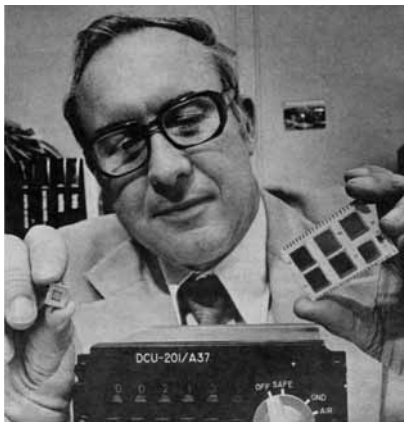
THE DCU-201 controller, the first PAL/AMAC controller to incorporate CMOS integrated circuits.
