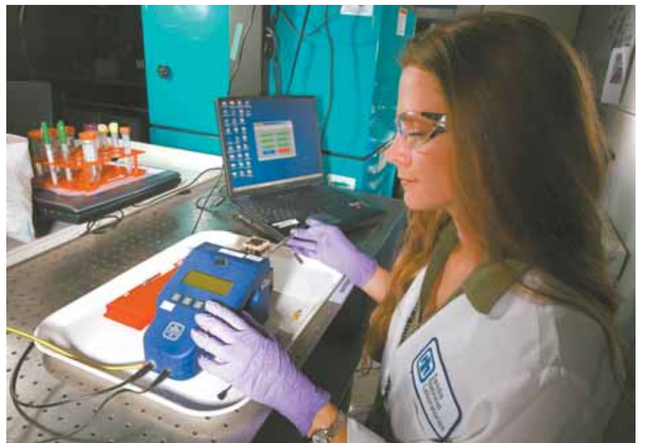
AMANDA JOKERST injects a sample into a handheld microseparations platform for analysis. Amanda and others at Sandia aim to optimize the microseparations process for a subset of relevant toxins found in harmful algal blooms and establish the laboratory-based protocols for sample preparation. (Photo by Jeff Shaw)
