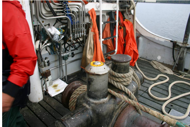
The “e-stop” mounted on the deck winch
