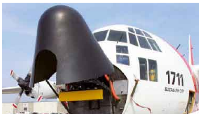
HC-130H with prototype APS-137 radar replacement (SELEX) installed
