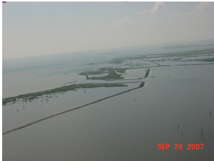
Aerial view of the interior (back) containment dikes that have been constructed to contain dredged material for the purpose of marsh creation. In order from front to back are the northern, central, and southern sections.
