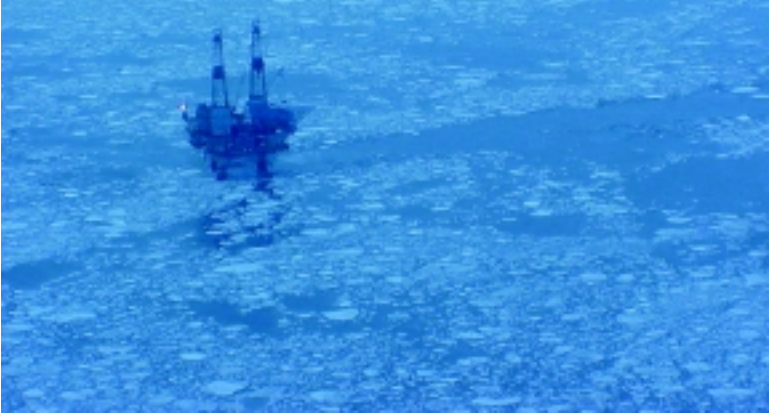
Ice Cake: Relatively level piece less than 20 m (65 ft) across (altitude 500 feet, Cook Inlet, Alaska)
