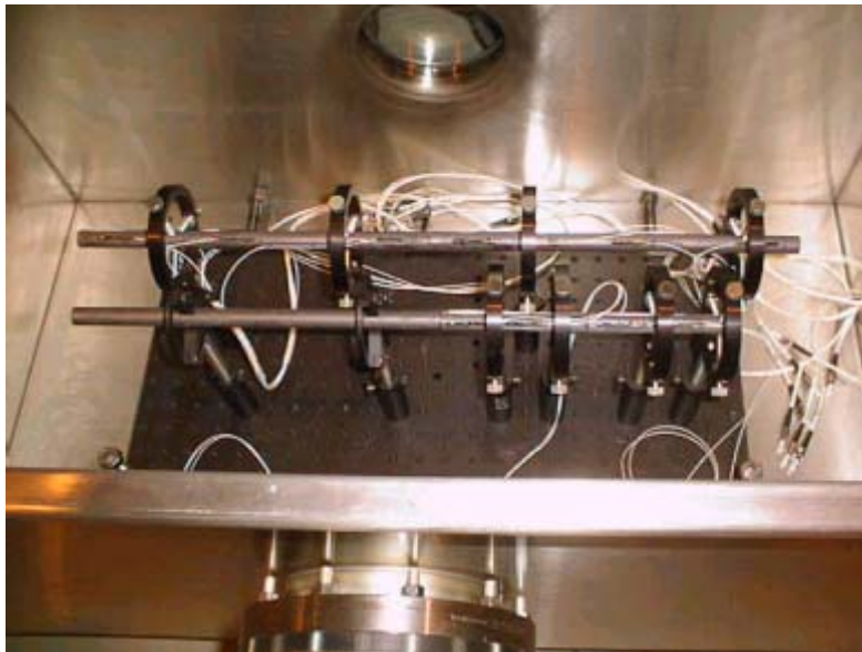
Figure 6.9: Carbon-Carbon composite and ATJ graphite target arrangement for the E951 experiment.
