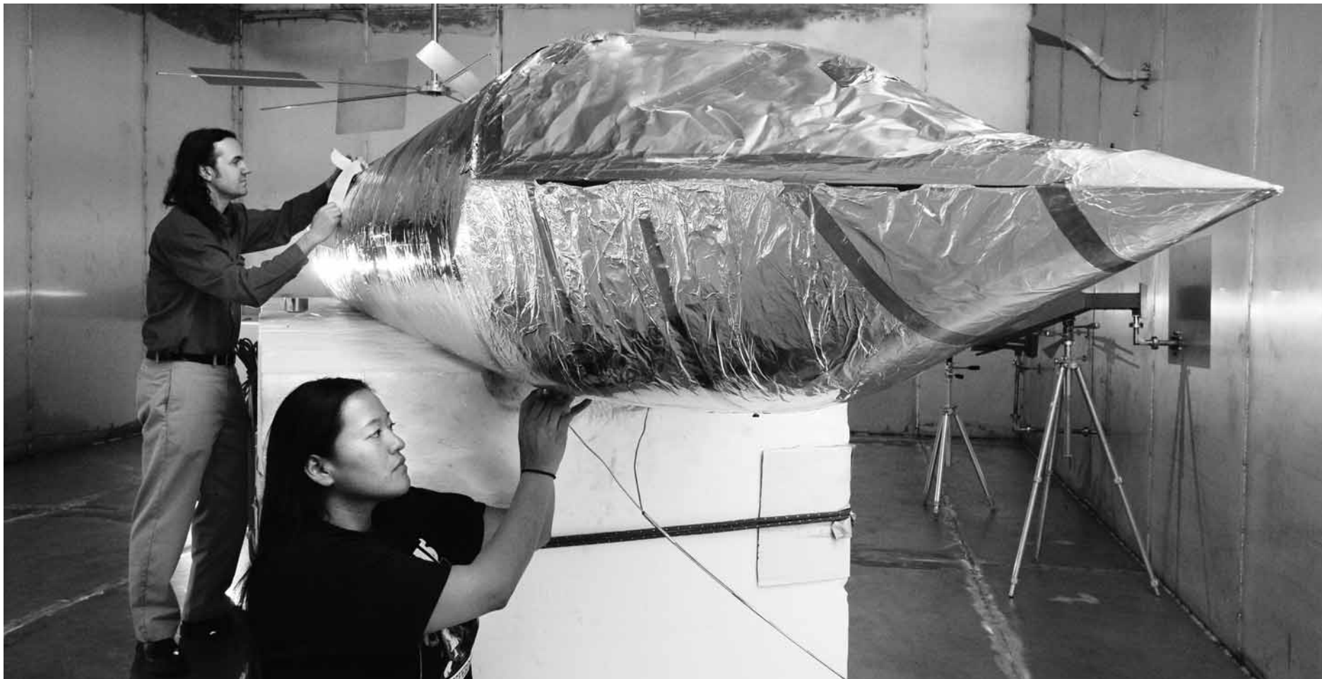
PROJECT LEAD Matthew Higgins (1653, left) conducts pre-test preparations, and Dawna Charley (1653) shows where measurements on two types of cruise missiles that carry the W80 have been performed in the Mode-Stirred Chamber. Other tests are performed in the Electromagnetic Environments Simulator. (Photo by Randy Montoya)
