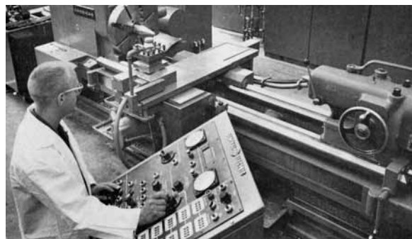
JOHN MALPAS using the manual override controls on the tape-controlled lathe.
