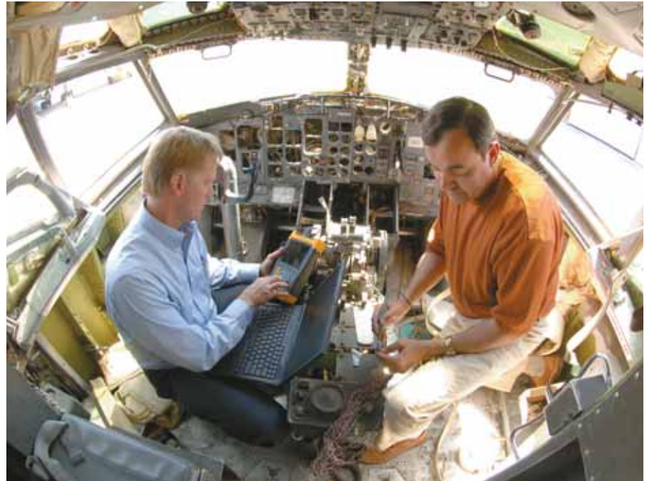
SPARKING THEIR INTEREST — Mike Dinallo and Larry Schneider (left) prepare to employ the PASD diagnostic on a wiring bundle in the cockpit of a retired Boeing 737 at Sandia's FAA Airworthiness Assurance NDI Validation Center.
