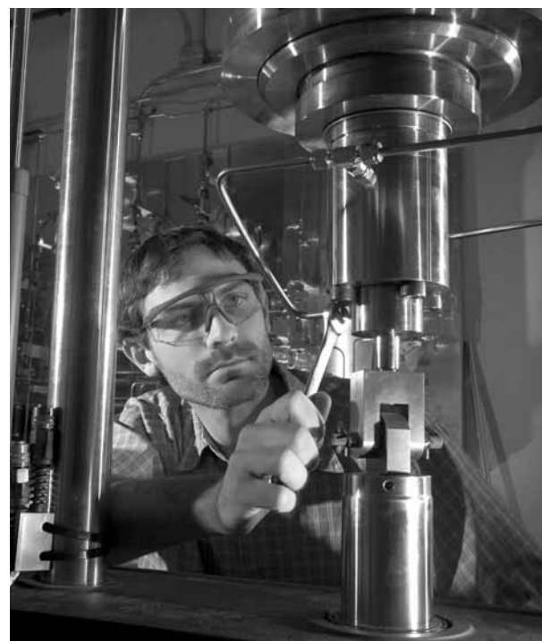
UNDER PRESSURE — To make it in the real world, containment materials first have to prove they have the right stuff in Sandia's high-pressure hydrogen test lab, which can reach pressures as high as 138 MPa (20,000 psi), a capability found in only two other labs in the world. Postdoc Kevin Nibur (8758) assembles a pressure vessel and pressure manifold on the mechanical test frame. (Photo by Randy Wong)
