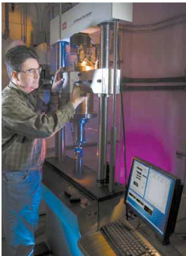
JUST SO — Ken Lee (8758) prepares the mechanical test frame to study how containment materials react to dynamic loads in high-pressure hydrogen gas. Sandia's high-pressure hydrogen test lab is the only one of its kind in the US (and only one of three in the world) with the capability to reach pressures as high as 138 MPa (20,000 psi). (Photo by Randy Wong)
