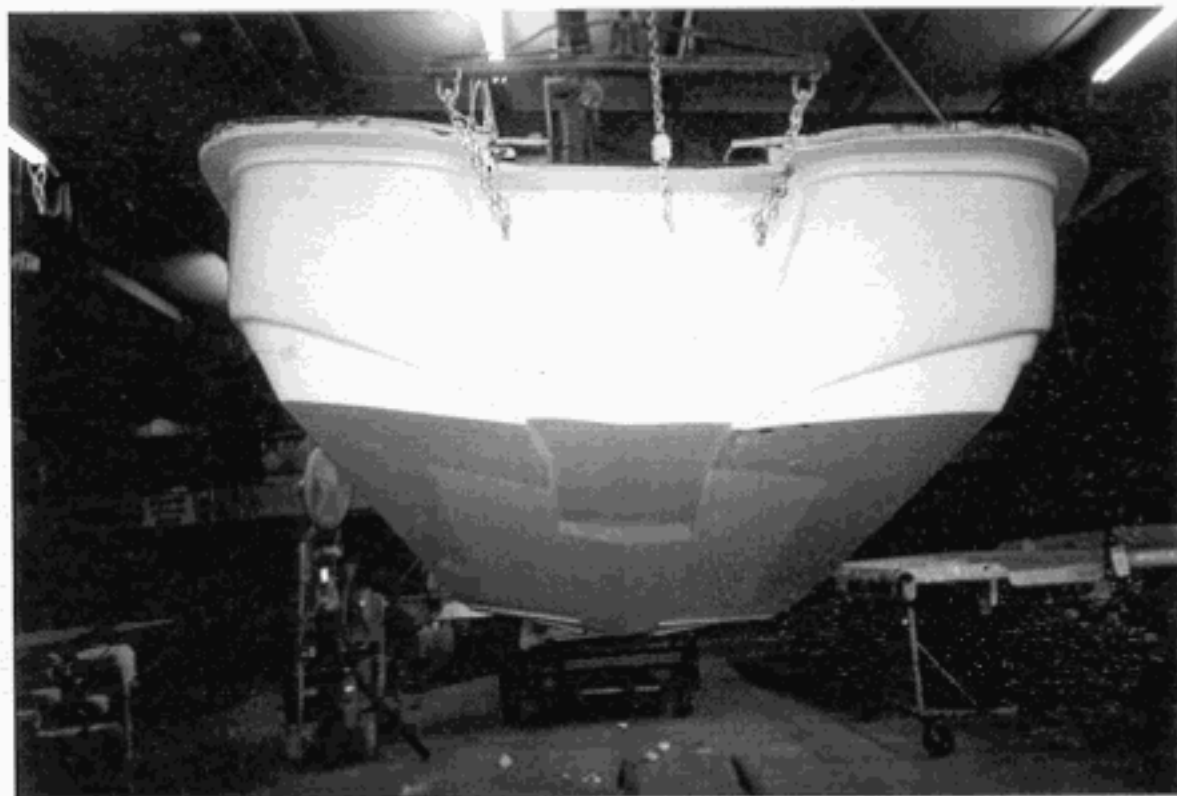
FULL STERN TUNNEL POCKET VIEW
