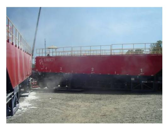
Figure 14 – Sand storage tanks.
