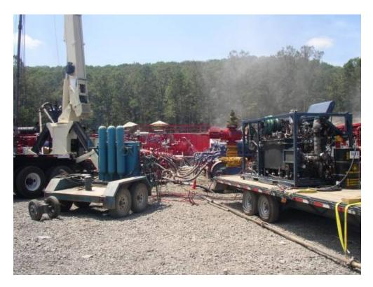
Figure 16 - The well being fracced is behind the white crane. The other wellhead near the middle of the picture was fracced on the previous day. In this case, two wells were constructed at the same well pad.
