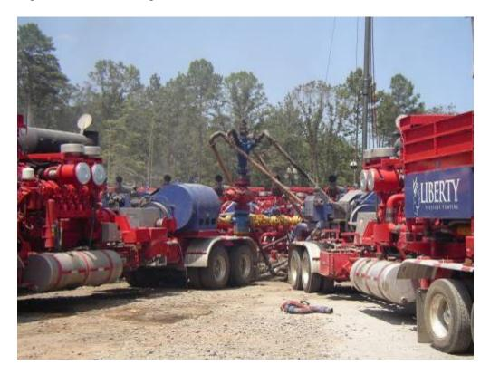
Figure 15 – The well being fraceed is in the middle, with the pipe conveying the injectate. The two trucks beside the well are pumping units.
