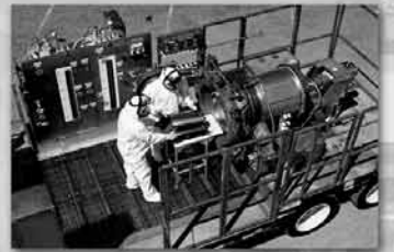
In 1998, Sandia delivered to the U.S. Army the Explosive Destruction System (EDS), which was designed to safely dispose of recovered chemical warfare materiel in an environmentally sound manner. A second phase EDS was delivered in 2003.
