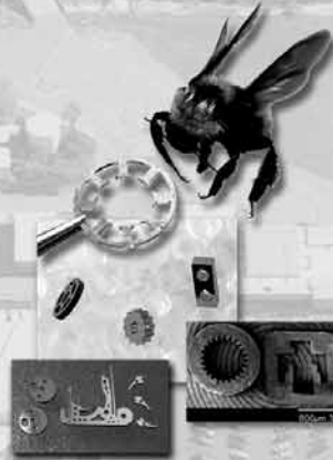
Sandia/California has led process development and fabrication of high-aspect-ratio micromachines for a variety of applications using LIGA technology (X-ray lithography, electroforming, and molding).
