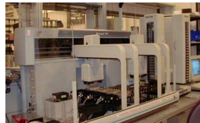
Biomek FX Liquid Handling Robot with Four 384-Well Hybrid Magnet Plates Installed
