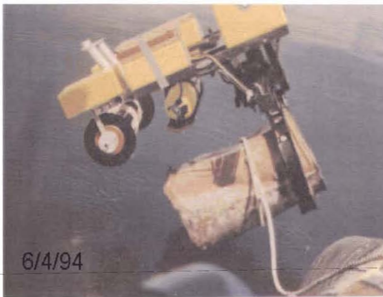
Photo 3A - Navy Torpedo Recovery ROV recovery of barrel from site 7.
