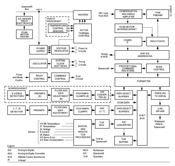
Figure 3-10. Imager Block Diagram
