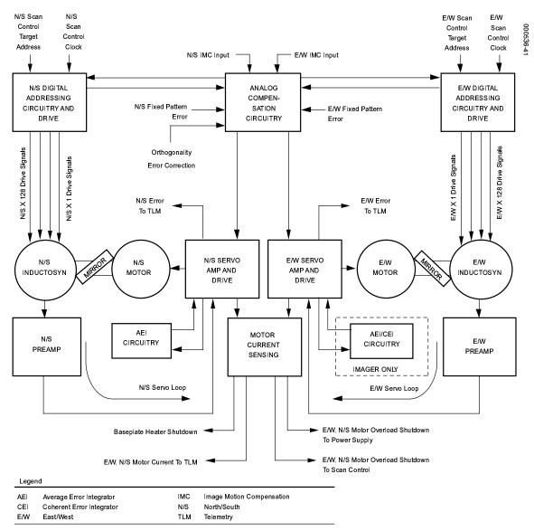
Figure 3-8. Scan Control Schematic
