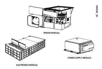
Figure 3-2. Imager Instrument Modules
