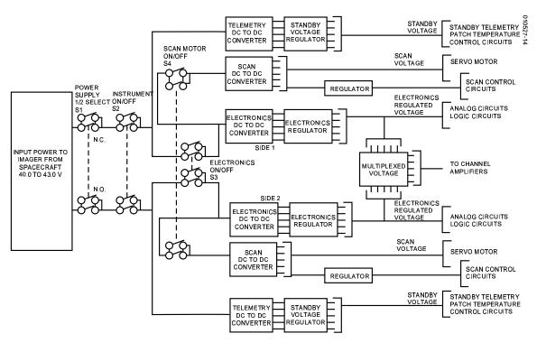
Figure 3-11. Power Supply Block Diagram
