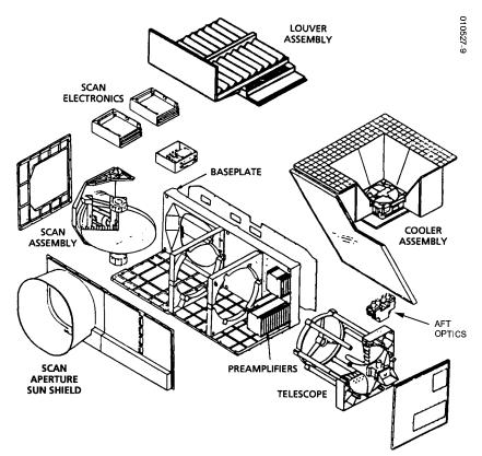
Figure 3-3. Sensor Module—Expanded View
