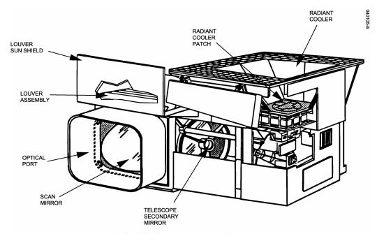
Figure 3-1. GOES N-P Imager Sensor Module
