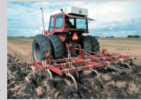
Deep chiseling improves water infiltration into the soil Photo: USDA
