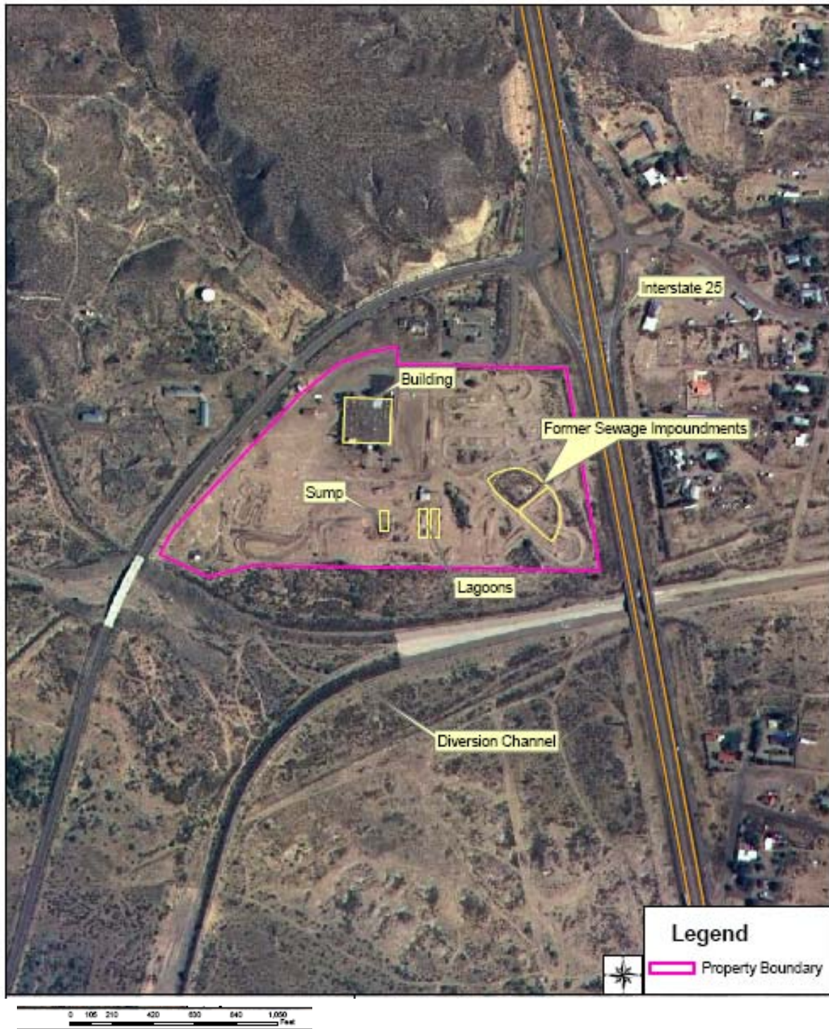
Figure 2. Aerial photograph of EP site and adjacent area showing locations of the sewage impoundments, former location of lined evaporation lagoons and main EP building. The former tuberculosis sanitarium and paintball course is immediately west of the property boundary. Note that the property outline of Figure 1 is much larger than the EP site boundary shown in this figure (from USACE, 2007).
