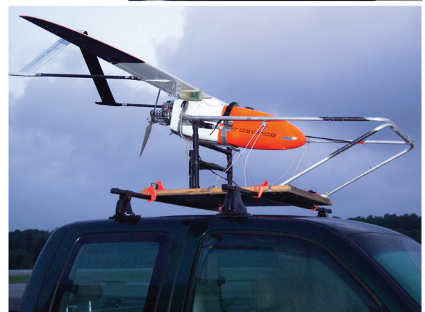
Images, top to bottom: A Remotely-Operated Vehicle is deployed during the Arctic 2005 Exploration; A Google Earth display of Global Ocean Observing System data; an Aerosonde® Unmanned Aircraft System is launched in Nov. 2007 from a moving platform to rendezvous with Hurricane Noel.
