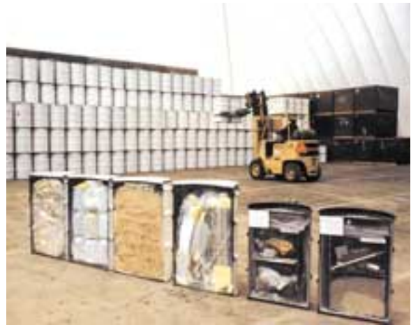
Cutaway of transuranic waste containers inside the air support building at Idaho National Engineering and Environmental Laboratory.
