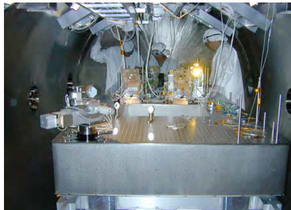
Fig. 28: Kite testbed in vacuum chamber.
