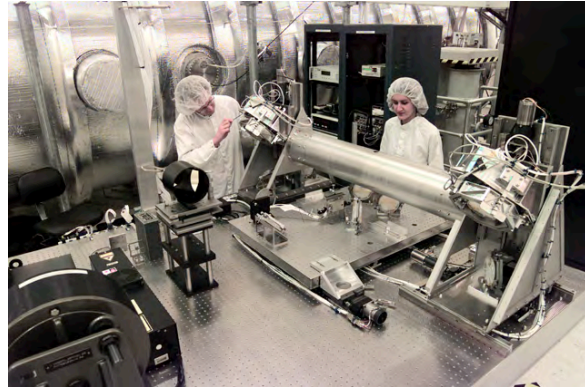
Fig. 22: MAM inverse interferometer pseudostar (IIPS) in final assembly
