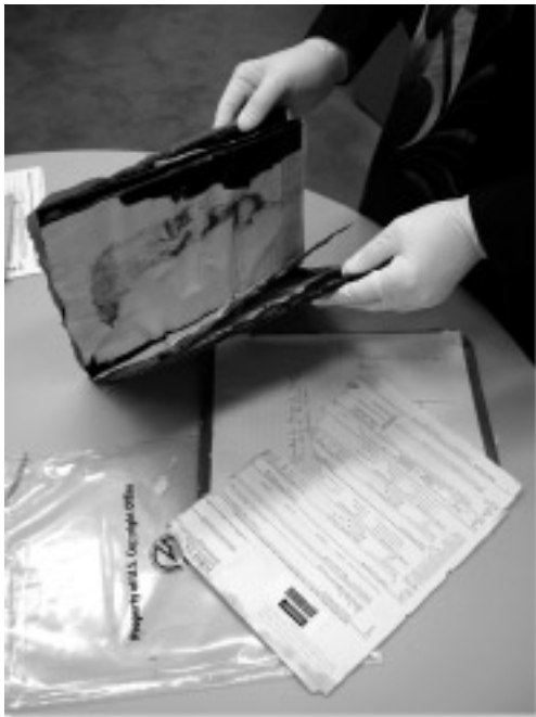
Irradiation of mail at offsite facilities damaged some materials submitted for copyright registration and deposit.
