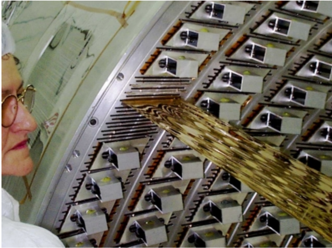
Installation of gold plated mylar field sheets in the Central Outer Tracker
