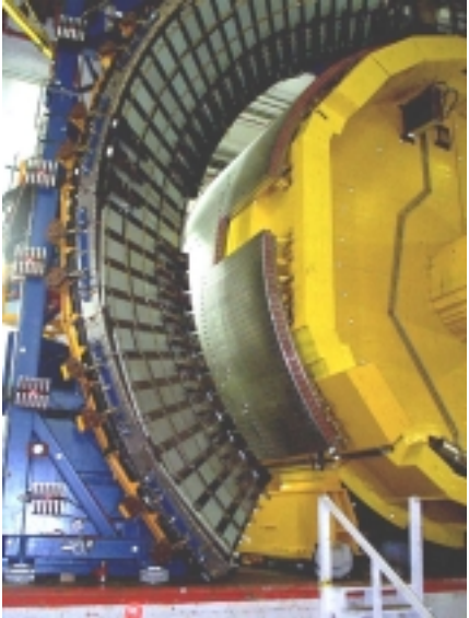
IMU chambers mounted on modified Toroid steel in collision hall.
