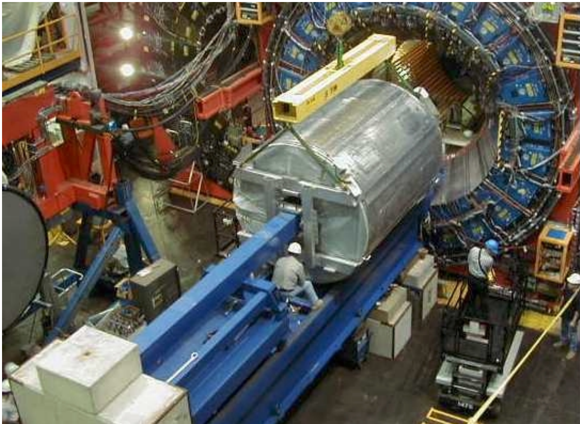
Installation of Central Outer Tracker
