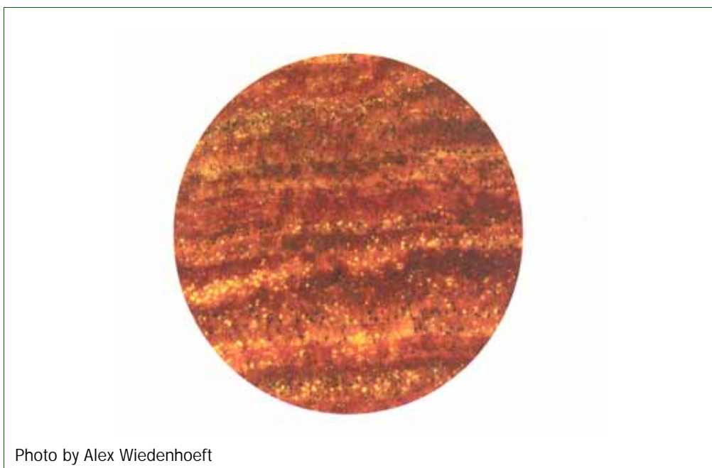
FIGURE F-11 Example of Guaiacum sanctum (Holy lignum vitae) Wood Cross Section
