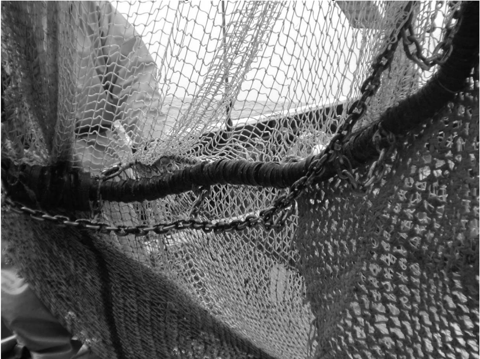
Exhibit 2. Canadian otter trawl showing footrope and tickler chain configuration.
