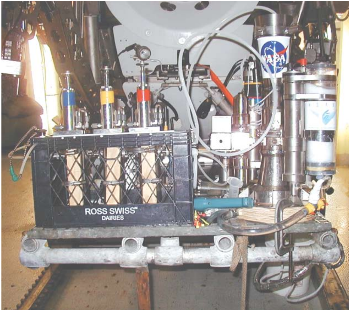
NASA's Medusa instrument inside the submergence vehicle Alvin's instrumentation basket in preparation for launch.
