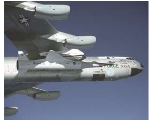
The first X-43A hypersonic research aircraft and its modified Pegasus booster rocket were carried aloft by NASA’s B-52 carrier aircraft from Dryden Flight Research Center on June 2, 2001, for the first of three high-speed free flight attempts.
