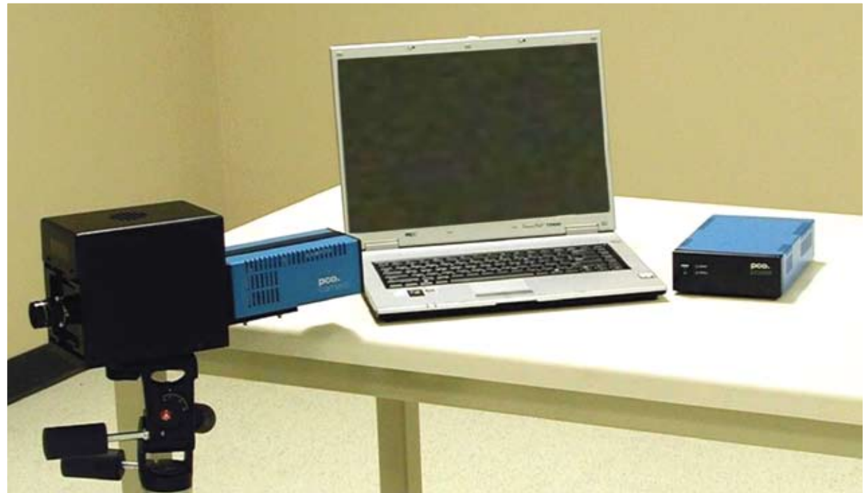
Lextel Intelligence Systems LLC made advances in the size, usability, and cost of the NASA-developed portable hyperspectral imaging instruments. The company now offers a suite of turnkey hyperspectral imaging systems based on the original NASA groundwork.
