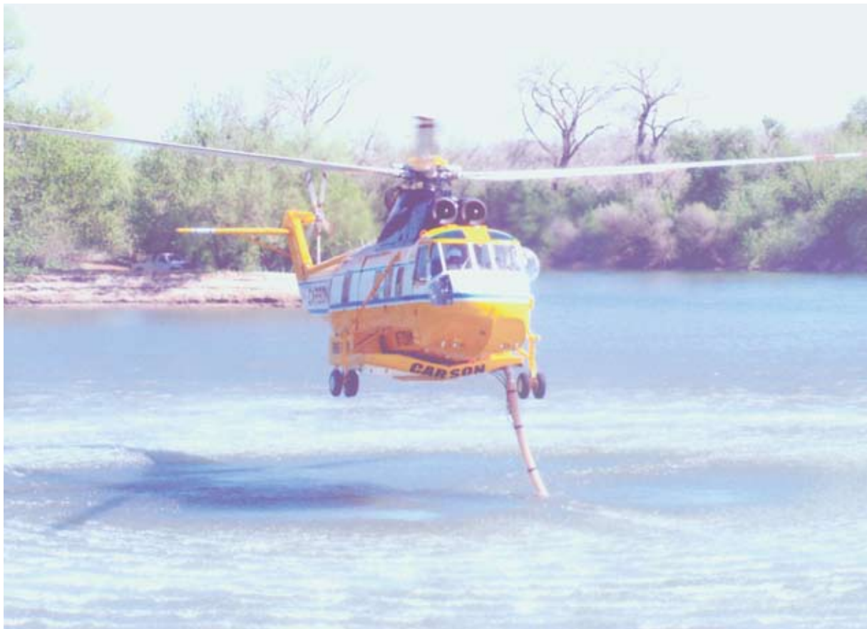
The NASA-developed rotorcraft airfoils permit greater lift and lower pitching-moments than other rotorcraft airfoils—ideal for heavy lifting operations.
