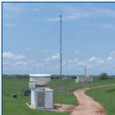
Cloud radars (foreground), a meteorological tower (background), and an aerosol observing system represent just a small portion of the remote-sensing instruments at the ARM Climate Research Facility's SGP site.
