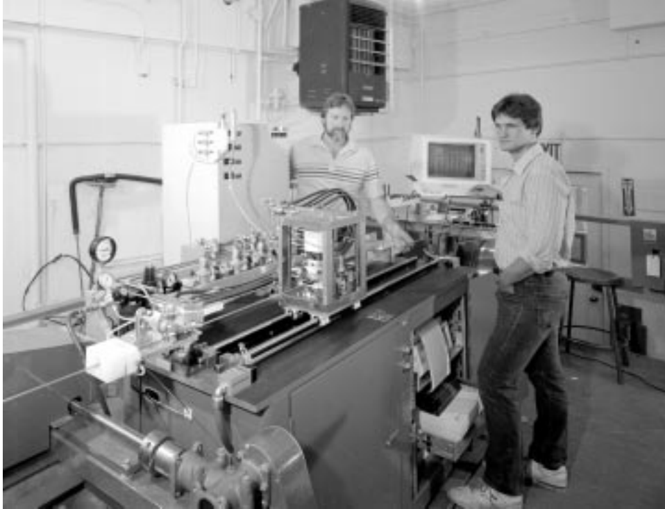
Fig. II.3.2.3-3. Photograph of a LBNL cable measuring machine (CMM).
