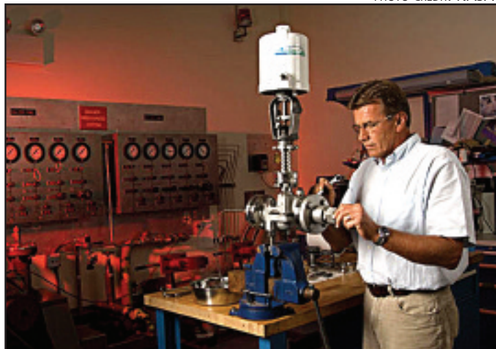
A CRYOGENIC GLOBE VALVE UNDERGOES DESIGN IMPROVEMENTS AND REFURBISHMENT IN PREPARATION FOR FUTURE LAUNCH PAD SERVICE.
