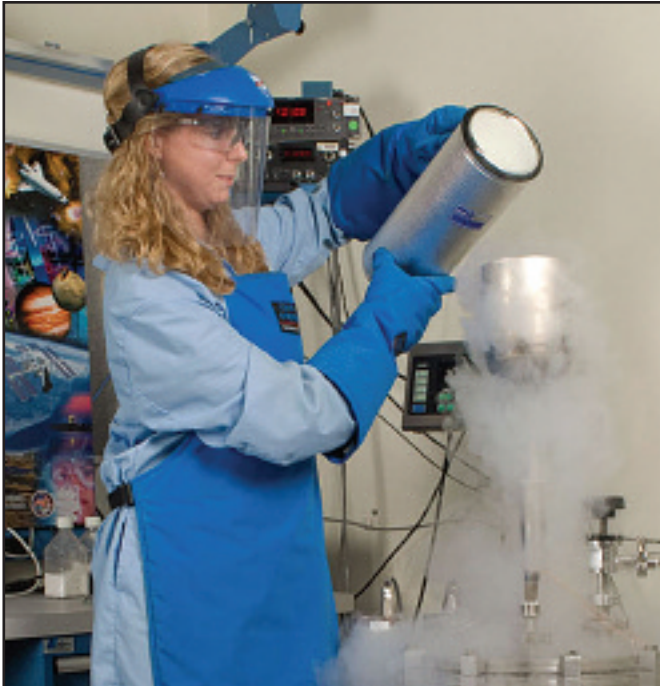
CRYOSTAT-4 (THERMAL INSULATION TEST APPARATUS FOR FLAT SPECIMENS) IS FILLED WITH LIQUID NITROGEN IN PREPARATION FOR TESTING NEW TECHNOLOGY MULTILAYER INSULATION SYSTEMS FOR FUTURE NASA EXPLORATION MISSIONS.
