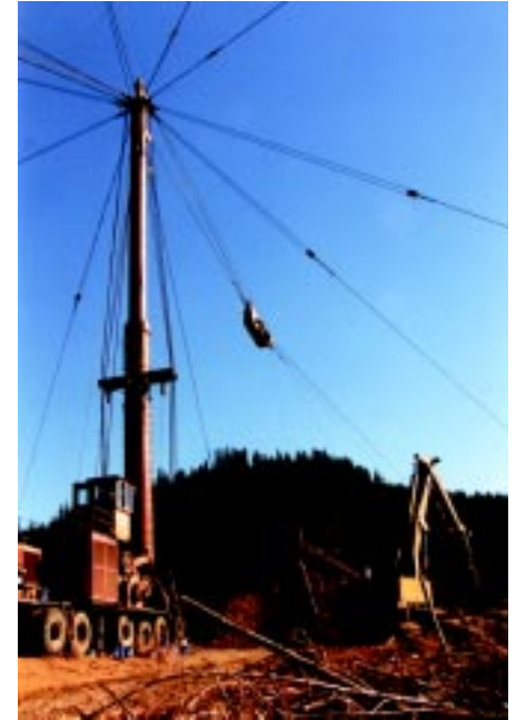
Northwest loggers use a cable yarding system to move logs from steep slopes.
