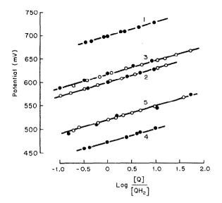
FIG. 1. Electrochemical potential at 25°C in 10% methanol/90% HCl/KCl as a function of the quinone (Q)/hydroquinone (QH<sub>2</sub>) concentration ratio. ◆, Quinone/hydroquinone mixtures; ○, quinone/ascorbic acid titrations. Curves: 1, p-benzoquinone; 2, methoxyquinone; 3, 2,3-dimethoxyquinone; 4, 2,5-dimethoxyquinone; 5, 2,6-dimethoxyquinone.
