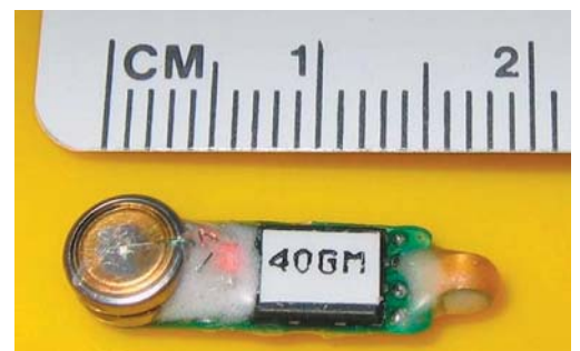
Mini-acoustic tag used to measure salmon survival
