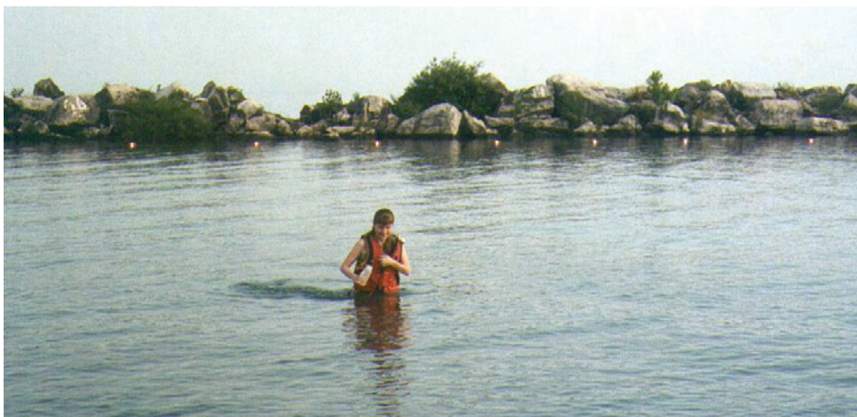
Samples are collected in a 500-mL autoclaved polypropylene bottle using a grab-sampling technique. (Photo by Donna Francy, U.S. Geological Survey.)
