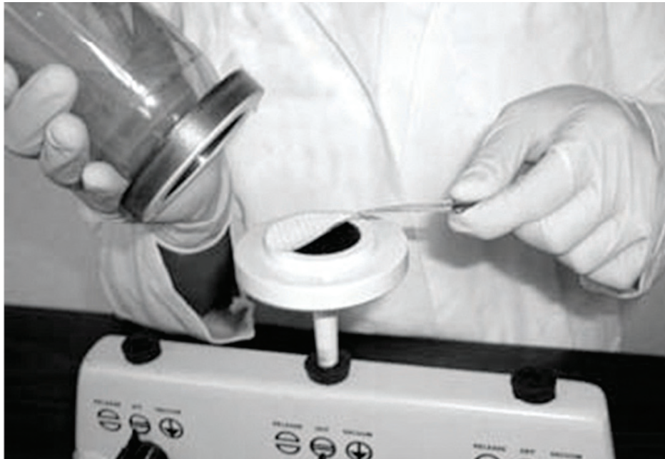
Filter being applied to suction device during membrane-filtration procedure. (Photo by Donna Myers, U.S. Geological Survey.)
