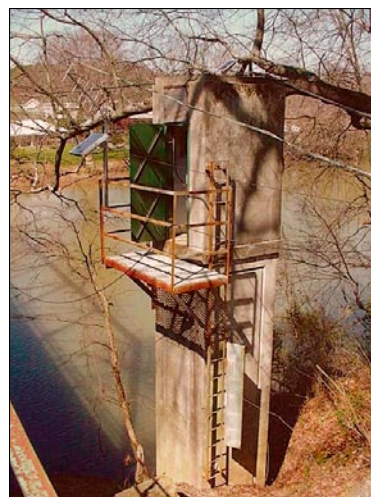
Real-time streamgage site is part of the USGS Hydrowatch Network. Several cooperators in Georgia provide funding for monitoring sites that collectively form a statewide real-time network of 222 streamgage and 19 ground-water sites (accessed on February 15, 2006, at http://ga2.er.usgs.gov/gawater/gawatersites.cfm ).
