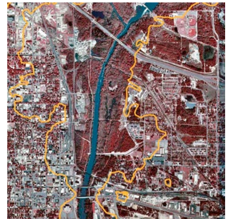
Digital orthophoto quadrangle showing extent of flooding at Albany from Tropical Storm Alberto during 1994. The USGS model, developed as part of the Cooperative Water Program, enables prediction of the extent of flooding under a wide variety of potential flood conditions (accessed on February 15, 2006, at http://ga.water.usgs.gov/pubs/other/gwrc2005/pdf/GWRC05_Musser.pdf ).
