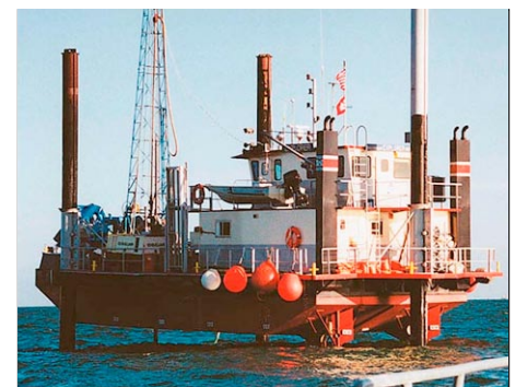
The U.S. Army Corps of Engineers jack-up barge was used as a platform for drilling offshore test borings as part of the Coastal Sound Science Initiative. Core, hydrologic, water-quality, and geophysical data were collected at five sites during 1999–2001. Data are being used to identify areas where saltwater is entering and contaminating the Upper Floridan aquifer, the principal source of freshwater in the coastal region. Photo by Michael F. Peck, USGS (accessed on February 15, 2006, at http://ga2.er.usgs.gov/coastal/ ).
