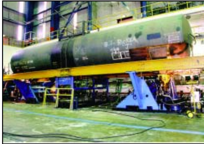
Tank Car NDE Inspection
