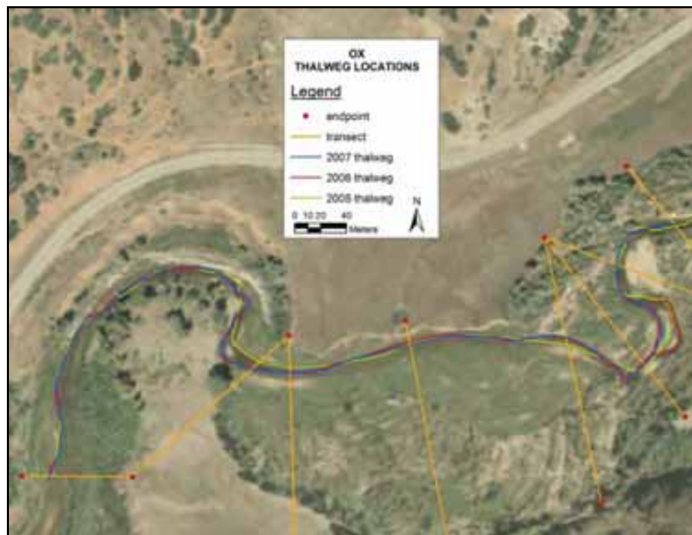
Figure 2.13. Location of the surveyed thalweg at the Oxbow (OX) site in 2005 and 2006 compared with 2007.
