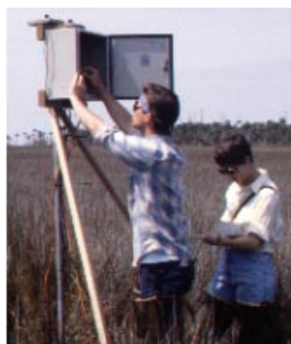
Fig. 1. Researchers monitoring salinity and water depth at St. Marks National Wildlife Refuge for comparison with satellite data.
