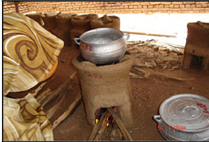
Photo 5.6: Six-brick stove, NGO C
