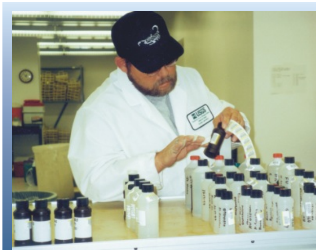
Sample login area is conveniently located near shipping and receiving. Samples are unpacked and bar-code labels are applied for identification and tracking.
