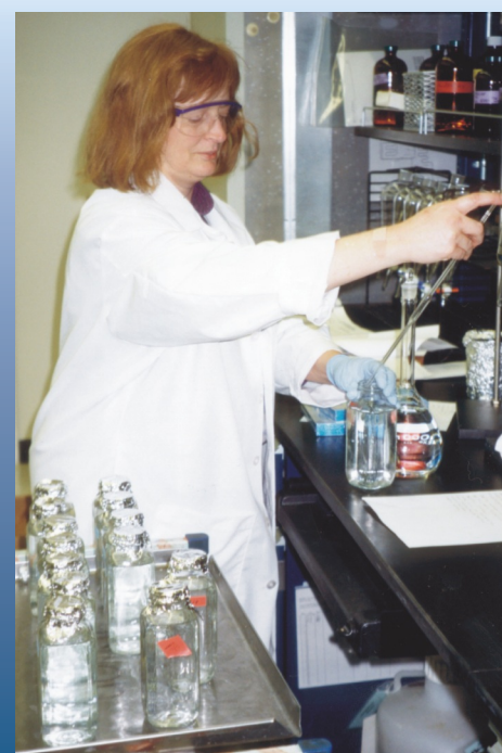
A spike is pipetted into a distilled water sample in the carbon lab.
