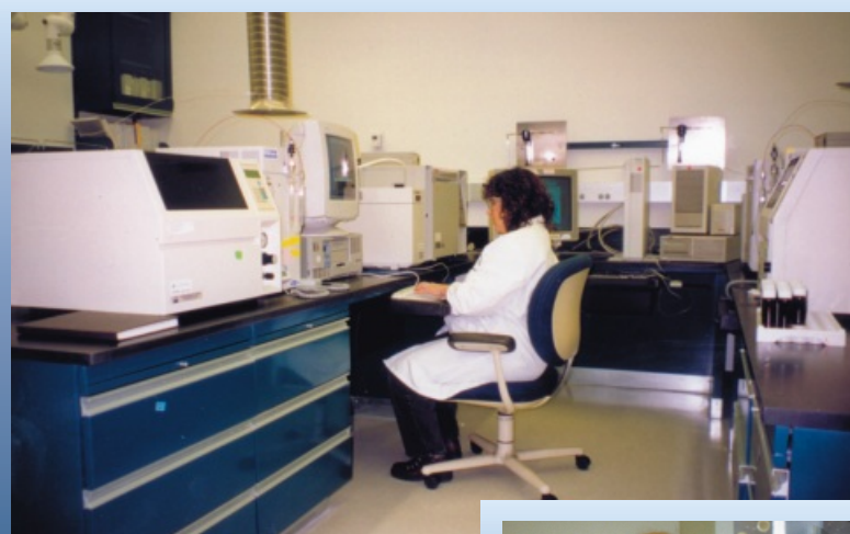
Gas chromatographic mass spectrometer is set up for determining presence and concentrations of volatile organic compounds.
