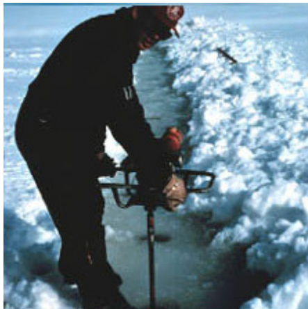
Left, a hydrologic technician drills through ice to measure stream flow. Photo Credit: U.S. Geological Survey.
