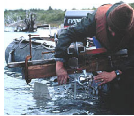
Left, a hydrologist prepares a current meter for stream measurement. Photo Credit: U.S. Geological Survey.
