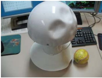
Hail damage to an Automated Surface Observing System (ASOS) from the Mississippidelta region
