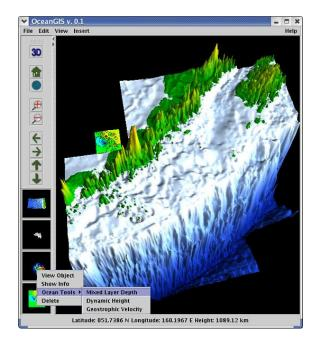
Figure 1 Tools for analyzing conductivity-temperature-depth data from the Bering Sea, Alaska
