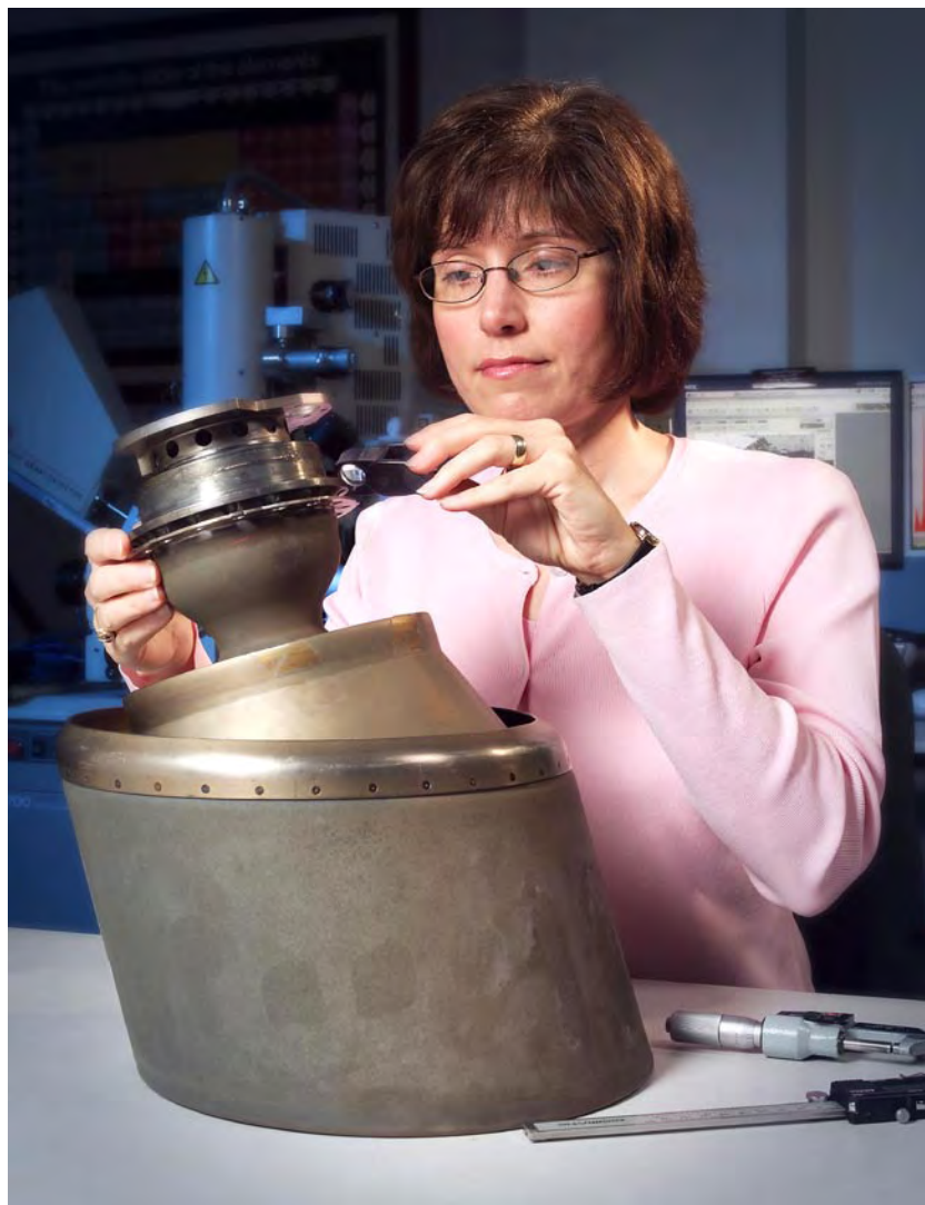
A thruster for the space-shuttle-orbiter reaction control system being examined in Glenn's Optics Laboratory.
