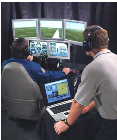
Pilot performing an approach to landing using the Ice Contamination Effects Flight Training Device, with an instructor observing pilot reactions.
