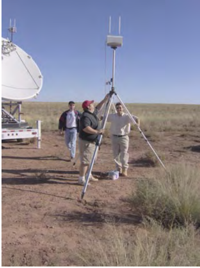
Glenn engineers and contractors deploying a surface proximity networking relay station during Arizona desert tests of Moon and Mars equipment.
