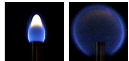
Video images of ethane jet diffusion flames in quiescent air. Left: 1g (Earth gravity). Right: \mu g (microgravity).
