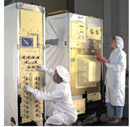
Systems and software engineers conduct final inspections of the Combustion Module 2 flight hardware at Glenn before it is shipped to the launch site.
