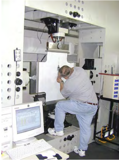
In-plane biaxial load frame with an ultrahigh strength fabric specimen mounted for a stretching test.
