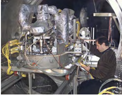
Closed-Brayton-cycle and NASA Solar Electric Propulsion Technology Application Readiness (NSTAR) thruster installed in Glenn's Vacuum Facility 6.
