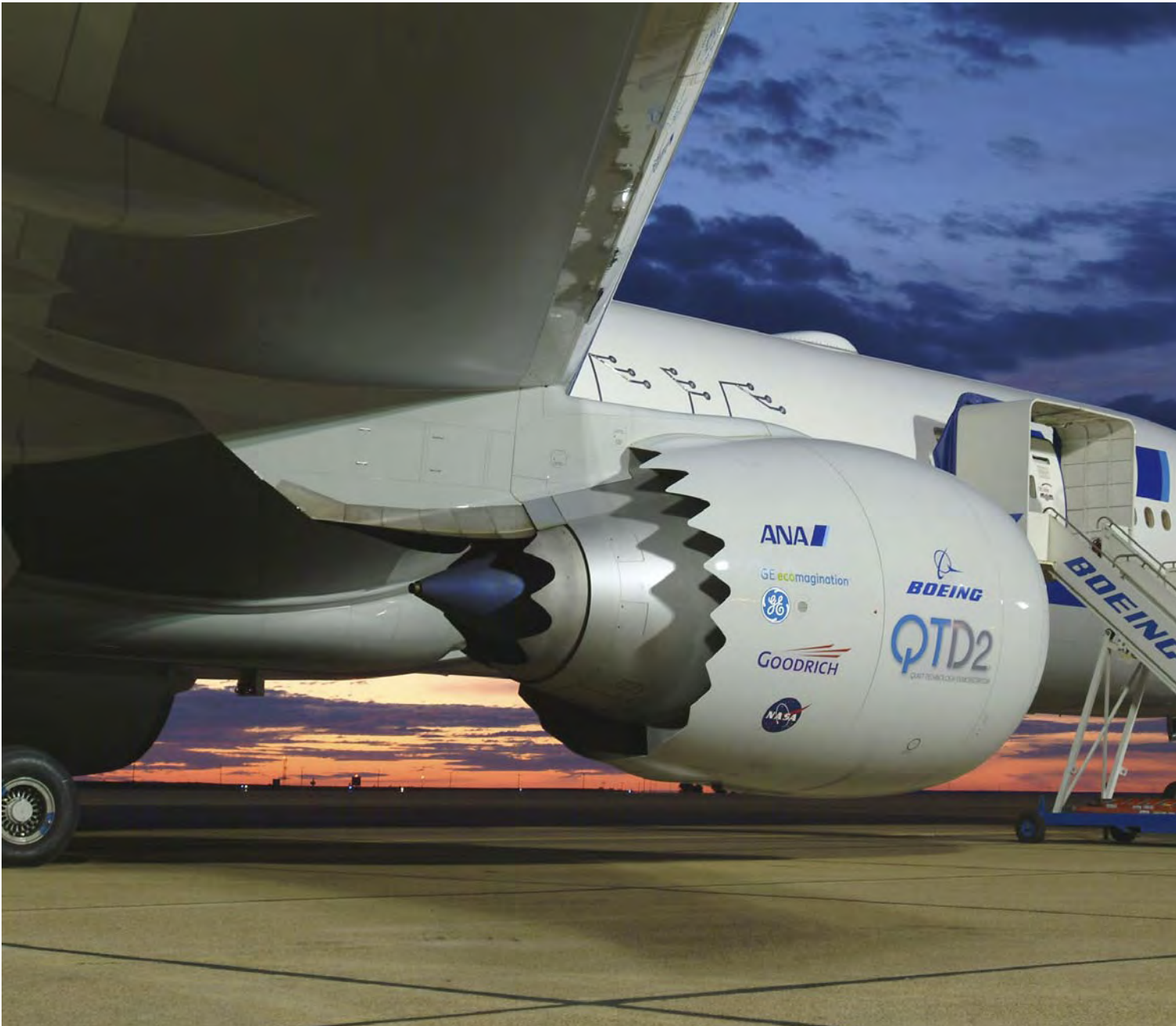
Glenn was the first to demonstrate more than a 50-percent reduction in jet engine exhaust noise using chevron nozzles in model-scale tests. Chevrons have subsequently been commercialized and tested on aircraft, as shown here on a GE90 engine on Boeing's 777 aircraft. (Copyright Boeing; used with permission.)
