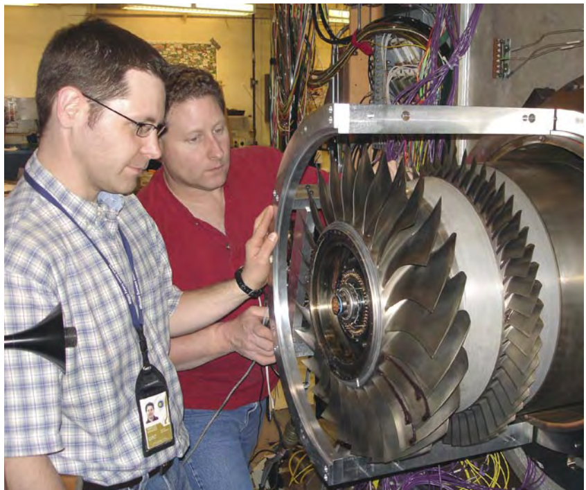
Ultra-Efficient Engine Technology (UEET) proof-of-concept compressor, a two-stage highly loaded compressor.
