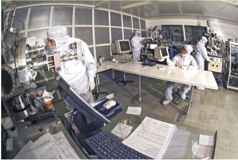
Glenn researchers fabricate microelectromechanical systems (MEMS) in this clean room. The air quality, humidity, and temperature are controlled to prevent contamination of sensitive material like MEMS.
