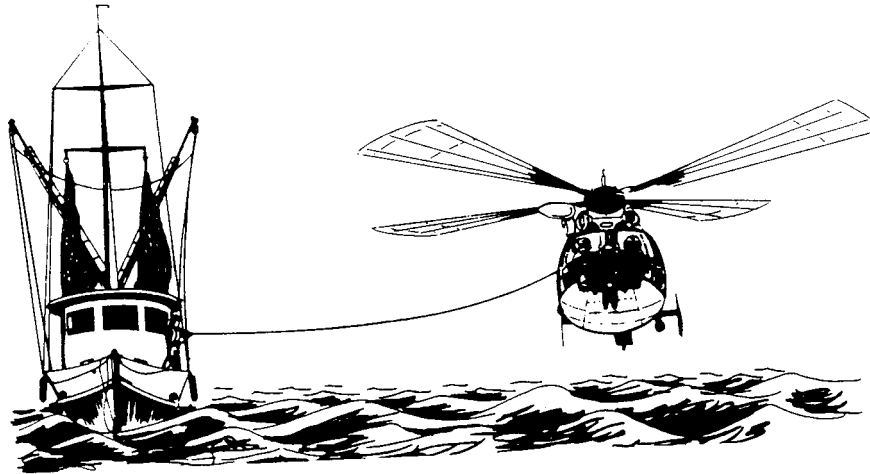
Figure 19-12 Indirect Delivery of Pump
