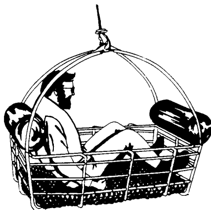
Figure 19-14 M/J Rescue Basket with Person Properly Positioned and Ready for Hoist
