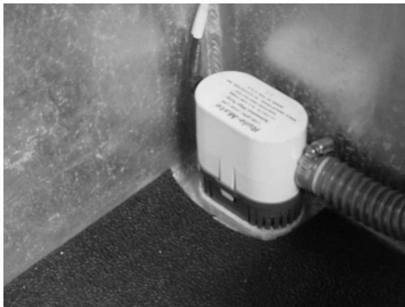
Figure 2-13 Electric Cabin Dewatering Pump (Defender B Class)
