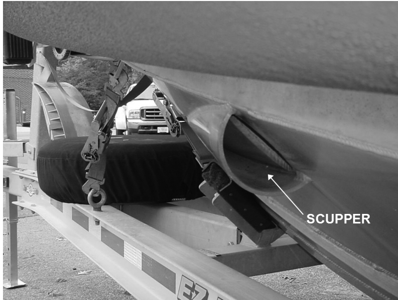
Figure 3-19 Forward Cabin Deck Scupper
