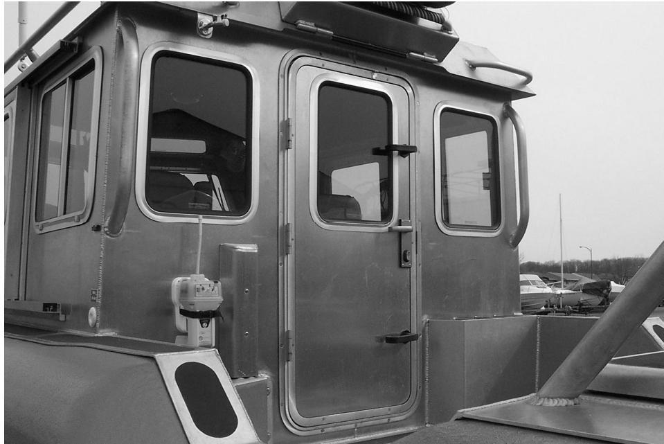
Figure 2-9 Aft Cabin Windows and Weather-Tight Door (Defender A Class)
